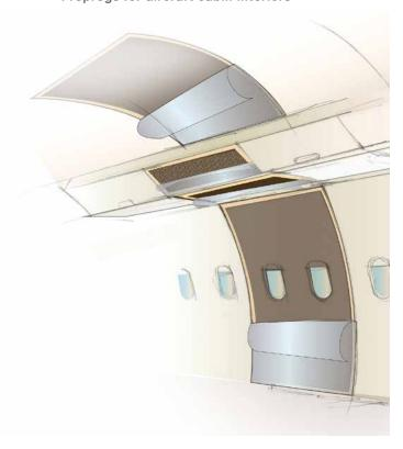
Thanks to the numerous combination options of material properties and their particularly low weight, composites are especially suited for use in aircraft interiors.
